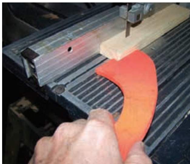
Figure 2-18. Keep fingers and hands away from cutting blades by using a push stick.
