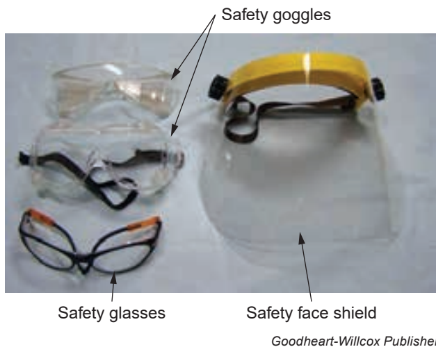
Figure 2-2. State and federal laws require the use of eye protection in the shop.
