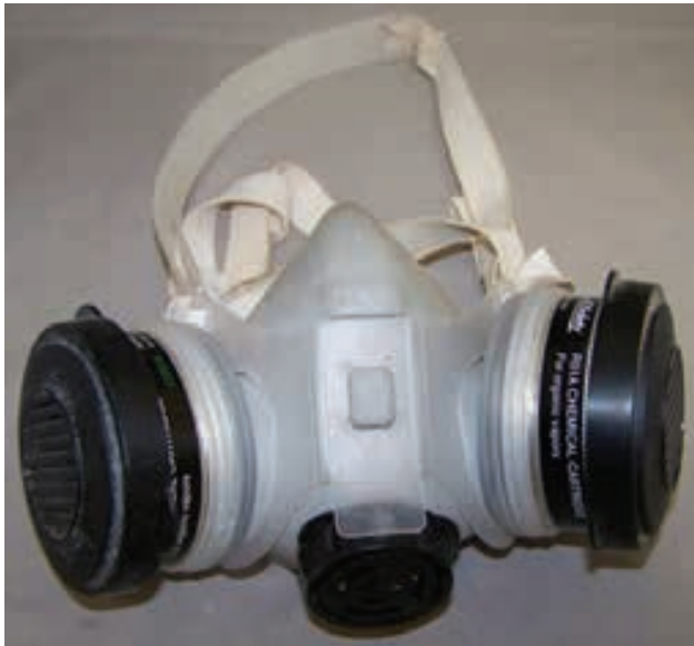
Figure 2-7. This NIOSH-approved respirator should be worn where there are fumes from wood finishing products.
