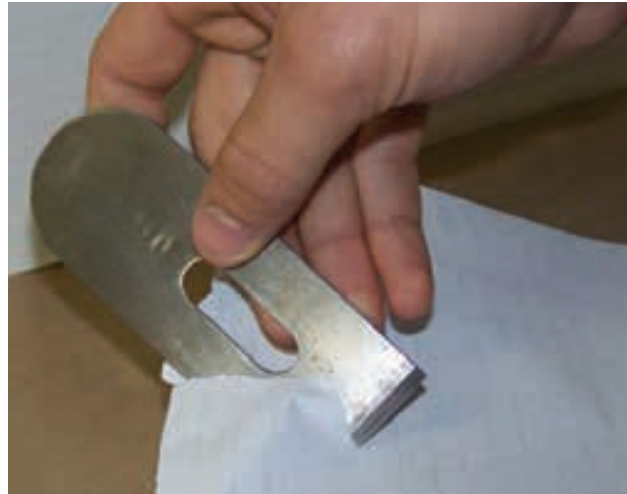
Figure 2-13. Make sure all cutting tools are sharp before using them.
