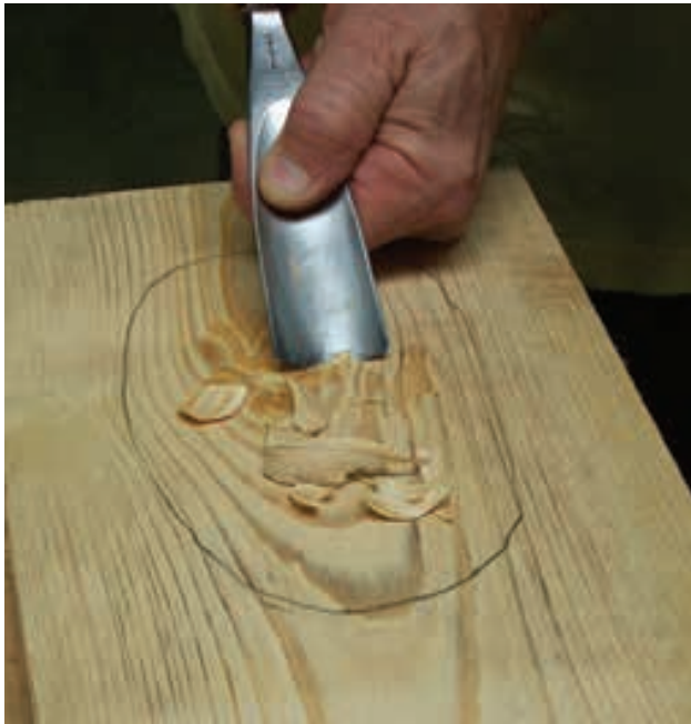
Figure 2-17. Cutting tools should be pointed away from the body.
