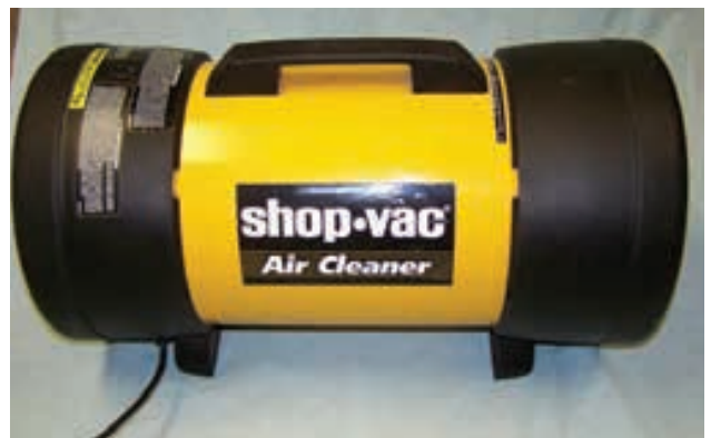
Figure 2-6. A portable dust collection device may be used if a larger system is not available.
