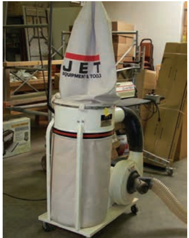
Figure 2-5. Most woodshops have commercial dust collection systems such as this one.
