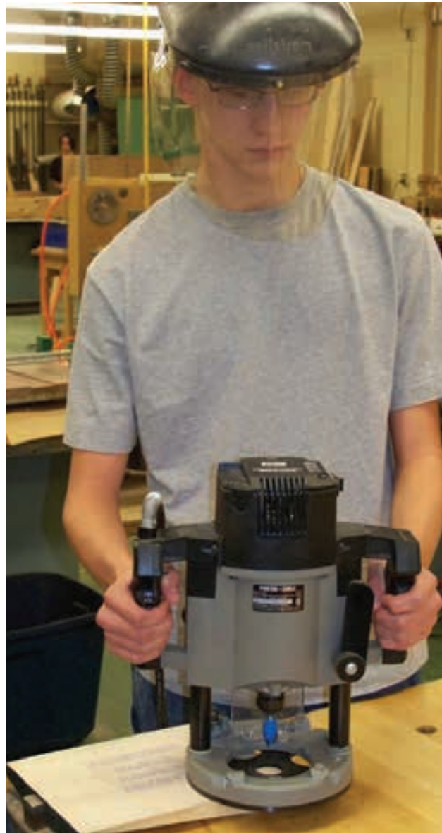
Figure 2-3. A safety face shield can be worn over regular eyeglasses.
